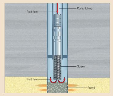
▲ Gravel pack washdown. As the gravel pack screen is lowered toward the top of the gravel, surface pumps are activated. The pump rate is sufficient to fluidize the gravel without causing it to circulate back into the tubing. While the pumps are active, the CT is slowly lowered into the gravel until the screen reaches its setting depth. A ball pumped through the CT string releases the screen before the CT string is pulled back to the surface.
