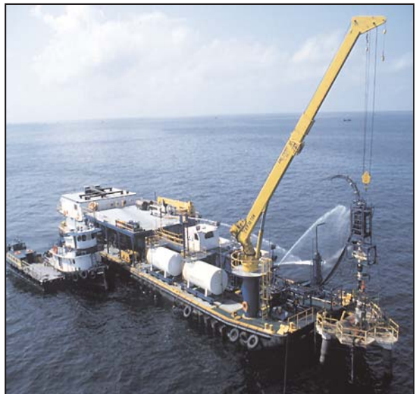
Figure 10: CT Operations from a Barge
