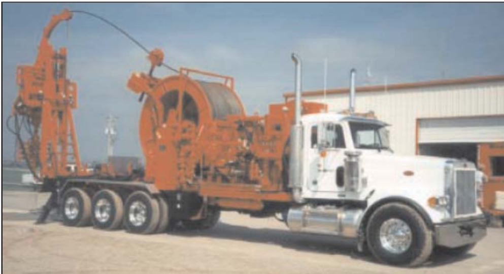
Figure 13: Truck Mounted 1 1/4in. CT Unit with Telescoping Hydra Lift for Fast Rigup
