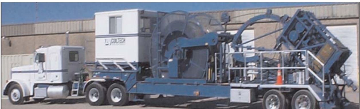
Figure 8: CT Unit Rigged Down for Highway Transport
